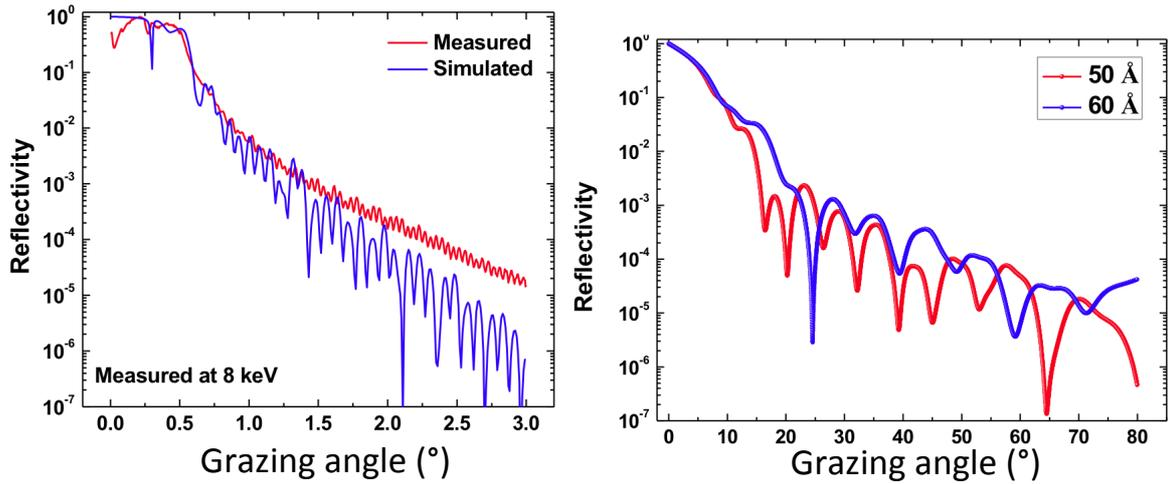
Figure 1 (left): XRR at 8.05 keV of the Al/ZrC/Al/W and the simulation obtained with a perfect stack with 0.5 nm roughness with the aimed thicknesses.
