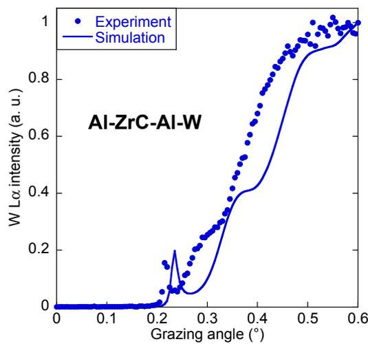
Figure 4: GIXRF of the W L $\alpha$  radiation excited at 10.25keV of the Al/ZrC/Al/W and the simulation obtained with a perfect stack with the aimed thicknesses.
