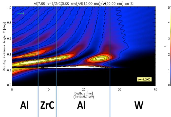
Figure 3: Depth and angular distribution of the electric field inside a Al/ZrC/Al/W waveguide excited by a 10.25keV radiation.
